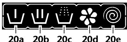
**i** At the beginning of every programme step, the corresponding symbol in the symbol array starts glowing and all of them go out together at the end of the programme. The right most glowing symbol in the array indicates the current step being executed.
