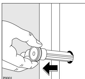
4. Place the machine in an upright position and remove the three plastic bolts.
